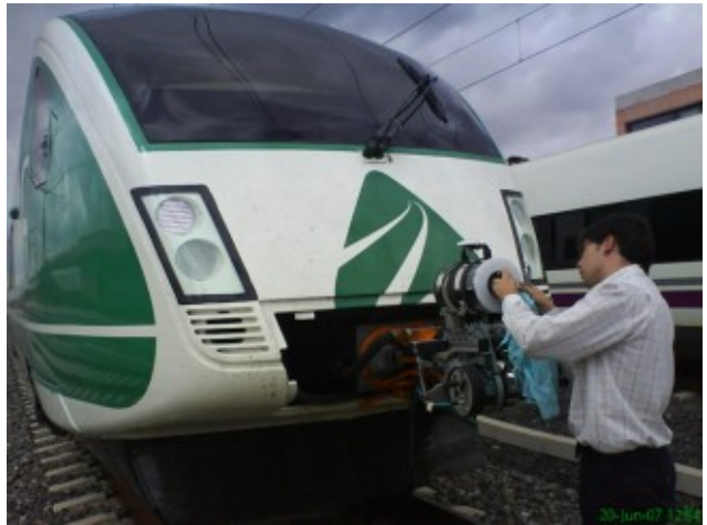
Installation of two LiDARs, video camera and GPS on the front of a high speed train modified for railway inspection
